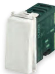
A compact device thanks to the integration of the Plana push button with the Quid magnetic relay for lighting control. It offers the possibility of creating a centralised power off control. Used to turn off all the lights with a single gesture. Moreover, the presence of a pilot light reveals whether the lighting is active in any point connected.
