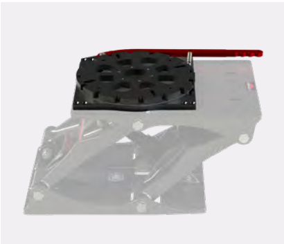
Swivel SW-05592 This robust 360-degree swivel is designed to pair with the S5 Sentinel and the Commander seat. A positive lock engages every 22.5° (16 positions).
