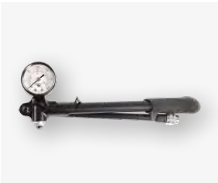
Shock Pump SW-01983 A Shockwave shock pump is required to operate the S5 Sentinel. The high-pressure shock pump features an integrated pressure gauge and bleed valve for simple adjustment with a maximum inflation pressure of 350 psi.
