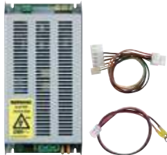
▲ 03806 230 V~ 50/60 Hz power supply unit with 13.8 Vdc 6.2 A output
