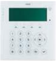
▲ 03818 Keypad with LCD display and transponder actuator, 2 In/Out zones/terminals, 12 Vdc, 23 backlit keys, 5 status LEDs, surface mounting. Dim. 140.3x150.3x21.6 mm
