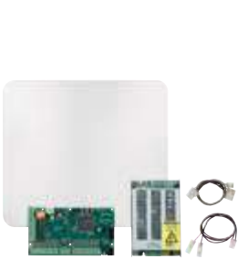
▲ 0K03800 By-alarm Plus control unit kit, 25 zones , surface mounting, containing: • 1 25-zone control unit board ( 03800 ) • 1 230 V – 13 Vdc 3.2 A power supply unit ( 03805 ) • 1 plastic box ( 03814 )
