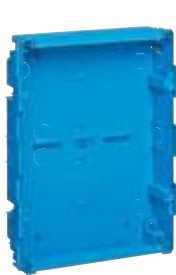
V53324 24-module flush-mounting back box (GW 650 °C) for masonry walls. Dim. 316x423x80 mm
