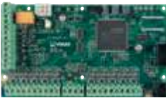
▲ 03801 By-alarm Plus control unit expandable to 65 zones
