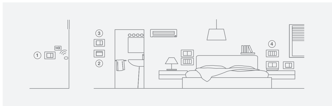
Inserting a card into the energy saver card switch switches on the electrical services.
