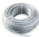
01841.E Bus system cable, 2x0,50 mm 2 , shielded, with LSZH sheath, CPR Eca class, suitable for I category cables (U0 = 400 V), for marine application, white - 100 m
