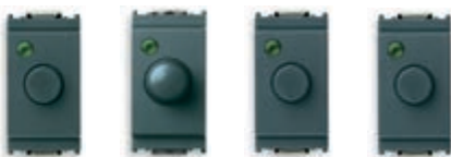
16560 100-500 W 230 V~ 50/60 Hz, potentiometer. Depth: 39,5 mm 16563 100-500 W 230 V~ 50/60 Hz, push-push and potentiometer. Depth: 39,5 mm *16556 60-900 W/ 60-300 VA 230 V~ 50/60 Hz, potentiometer. Depth: 39,5 mm 16557 30-500 W/ 30-300 VA 120 V~ 50/60 Hz, potentiometer. Depth: 39,5 mm
