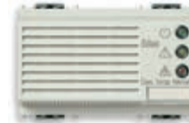
16592.B Gas Stop Metano, methane detector, solenoid valve control, 230 V~ - 3 modules. Depth: 42,5 mm
