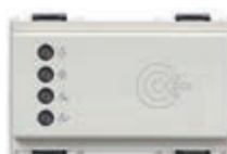
16927.B Transponder card reader for installation outside rooms, KNX standard, 2 NO 4 A 24 V~ relay outputs, 2 inputs, power supply 12-24 V~ 50/60 Hz and 12-24 Vdc (SELV) - 3 modules. Supplied without transponder card. Depth: 36,5 mm
