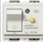
16511.06.B C 6, I_{\Delta n} 10 mA, breaking capacity 1500 A - 2 modules. Depth: 38 mm
