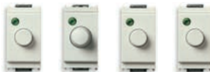
16560.B 100-500 W 230 V~ 50/60 Hz, potentiometer. Depth: 39,5 mm 16563.B 100-500 W 230 V~ 50/60 Hz, push-push and potentiometer. Depth: 39,5 mm *16556.B 60-900 W/ 60-300 VA 230 V~ 50/60 Hz, potentiometer. Depth: 39,5 mm 16557.B 30-500 W/ 30-300 VA 120 V~ 50/60 Hz, potentiometer. Depth: 39,5 mm
