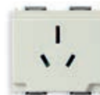
16262.B SICURY 2P+E 15 A, Australian - 2 modules. Depth: 26,5 mm
