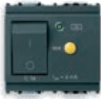
16511.16.6 C 16, I_{\Delta n} 6 mA, breaking capacity 3000 A - 2 modules. Depth: 38 mm
