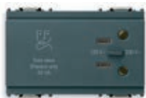
16290 230 V~ 50/60 Hz, with isolating transformer 20 VA, 230 V~ and 120 V~ outputs - 3 modules. Depth: 46 mm
