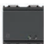
16975 Actuator, 16 A 120-230 V~ change-over relay output - 2 modules. Depth: 36,5 mm
