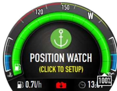
To **enable** the function: navigate to the Position Watch screen, after a short click on the Jog wheel the following screen will appear:
